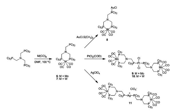
Scheme 2. Reaction of the dicyclohexylphosphine N-triphos ligand (4) with Mo(CO)<sub>6</sub> and W(CO)<sub>6</sub>, followed by coordination of the free phosphine arm to form a series of heteromultimetallic gold, platinum and silver complexes.
